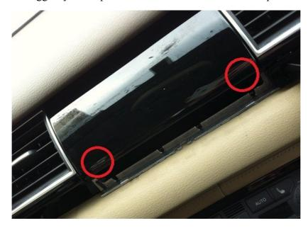
4. Remove the rightmost AC vent by lifting up the 2 lugs at the bottom with a pointy object. This can be a little frustrating but don't give up...Wiggle it out and disconnect. Behind this trim is an Allen 4 screw that must be removed. To facilitate potential future operations you can skip this one when refitting the trim later.
