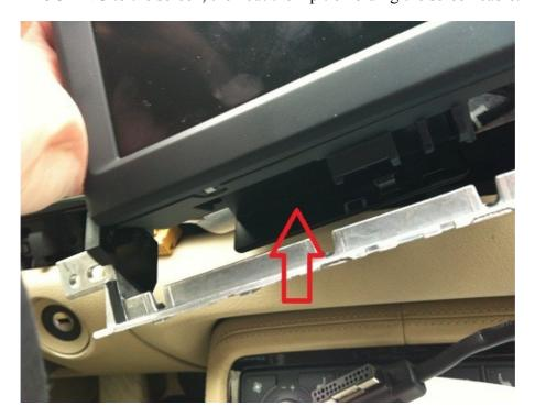
9. To avoid removing the small cable harness from the frame you can unplug it instead. To the right of the ignition, you will be able to feel the connector. It sits to the panel with a "plug" so you will need to wiggle it out of the hole. Then disconnect, remove the "plug" and pull out the connector from the MMI side. It's a bit tight so take it easy.
