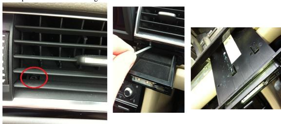
5. One torx for the "quattro trim" sits behind the storage compartment so it must be removed. Either remove the vent above it per above instruction or you can also insert a thin object on top of it, carefully press down on it and it should be possible to pull out. Disconnect.
